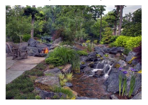
**6.)** Impressive bluestone patio slabs meet the boulder firepit. The larger bluestone slabs were painstakingly assembled by chiseling the stone to ensure a natural feel and proper placement. The boulder firepit also serves as a retaining wall to support the grade change needed for the stream.
